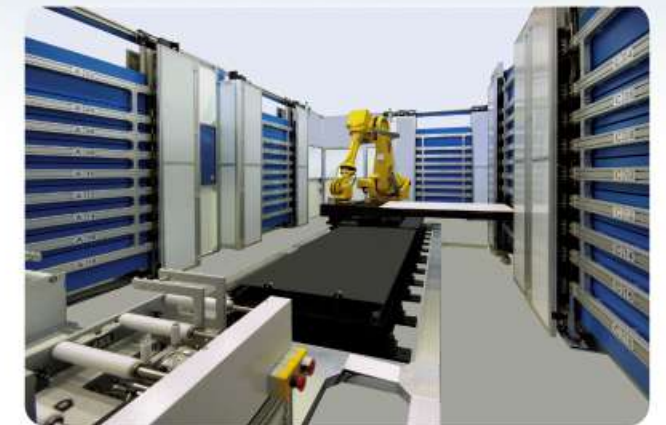
熱板熱風多層爐 Auto Multi Layer Oven ● TFT LCD Seal Main Cure / Annealing / ARCO / PIPB製程烘烤 ● 太陽能EVA固化烘烤
