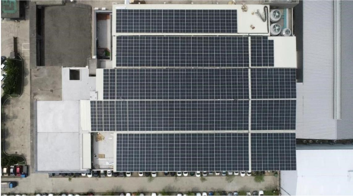
日均發電量 =  $0.37\text{kW} \times 1340(\text{片}) \times 2.9\text{hr} = 1437.82\text{kWh}$  ( $1\text{kW} \times 1\text{hr} = 1\text{度}$ )
